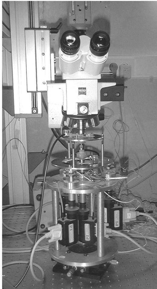
FIGURE 2 Schematic of the microtack tester with microscope viewing capability.
